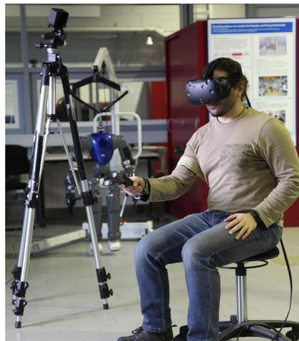
Fig. 1. User equipped with Head Mounted Display and controllers performing the virtual ball catching task.
